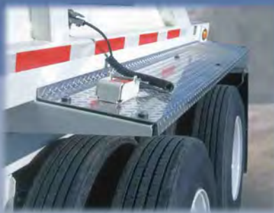
Full-Width Aluminum Fenders, both front and rear, are sloped to shed material more effectively.
